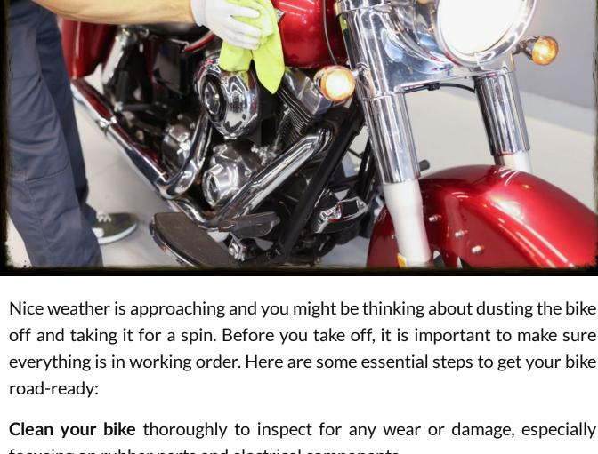
focusing on rubber parts and electrical components. Check your tires for cracks, abnormal swelling, and inspect the tire date codes. Consider replacing tires that are three to five years old. Clean and inspect the final drive, including the chain and sprockets. Replace
